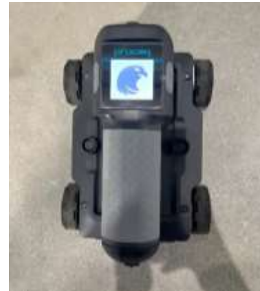
Figure 4. Proceq GP8000 GPR
