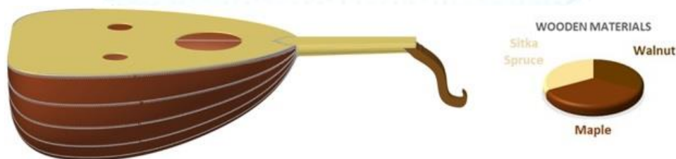
Figure 6. The orthotropic wooden materials assigned to the FE model of oud guitar
