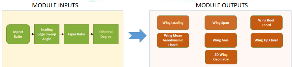
Figure 7. Inputs and Outputs of Module 2 / Wing Selection Submodule
