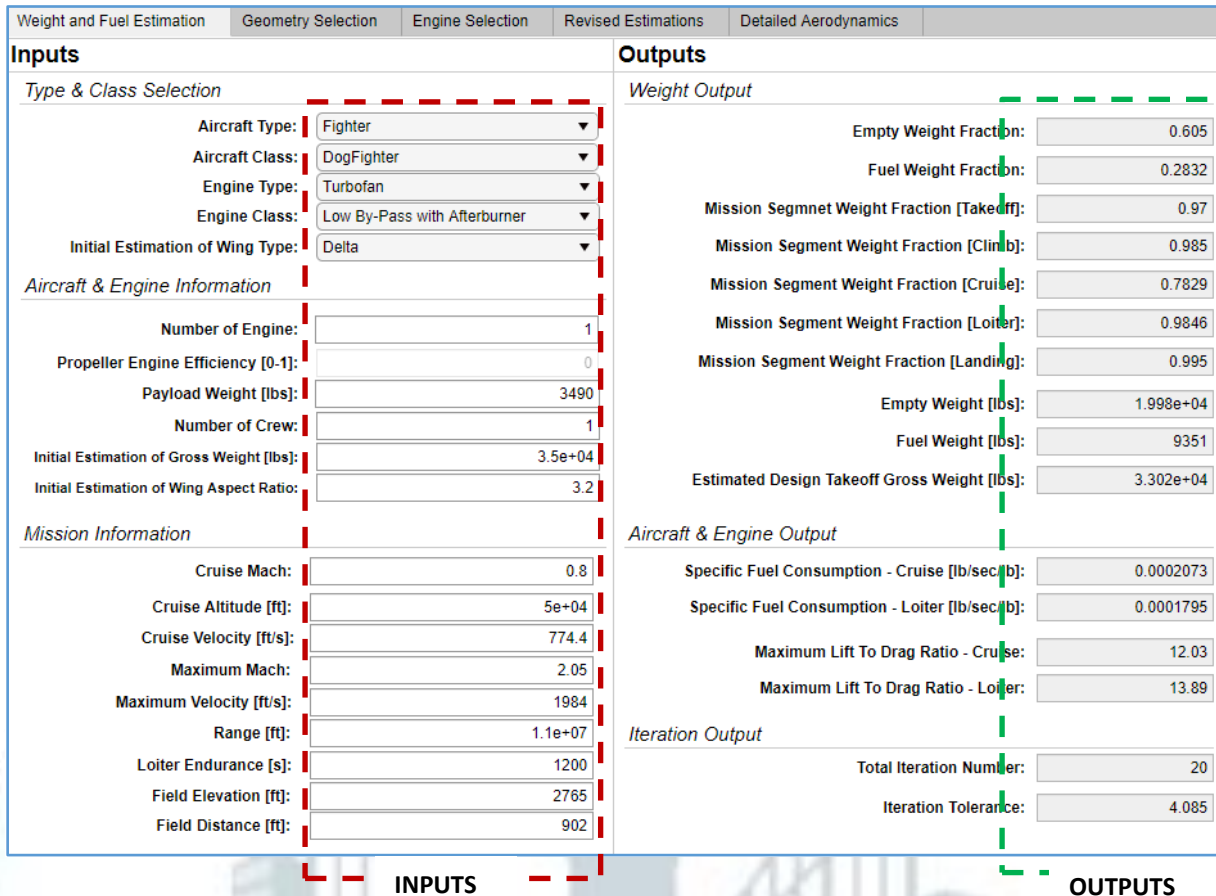
Figure 13. F-16 Real Data and HAKTAS Outputs (Module-1)
