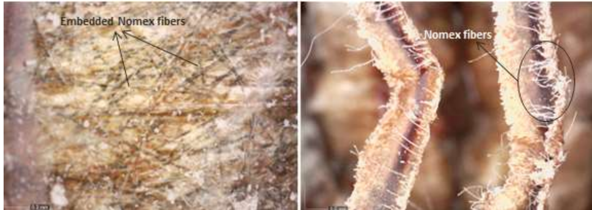
Figure 12. Embedded Nomex fibers in Nomex paper
