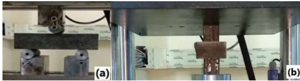
Figure 4. Flexural Strength (a) and Compressive Strength (b) Tests
