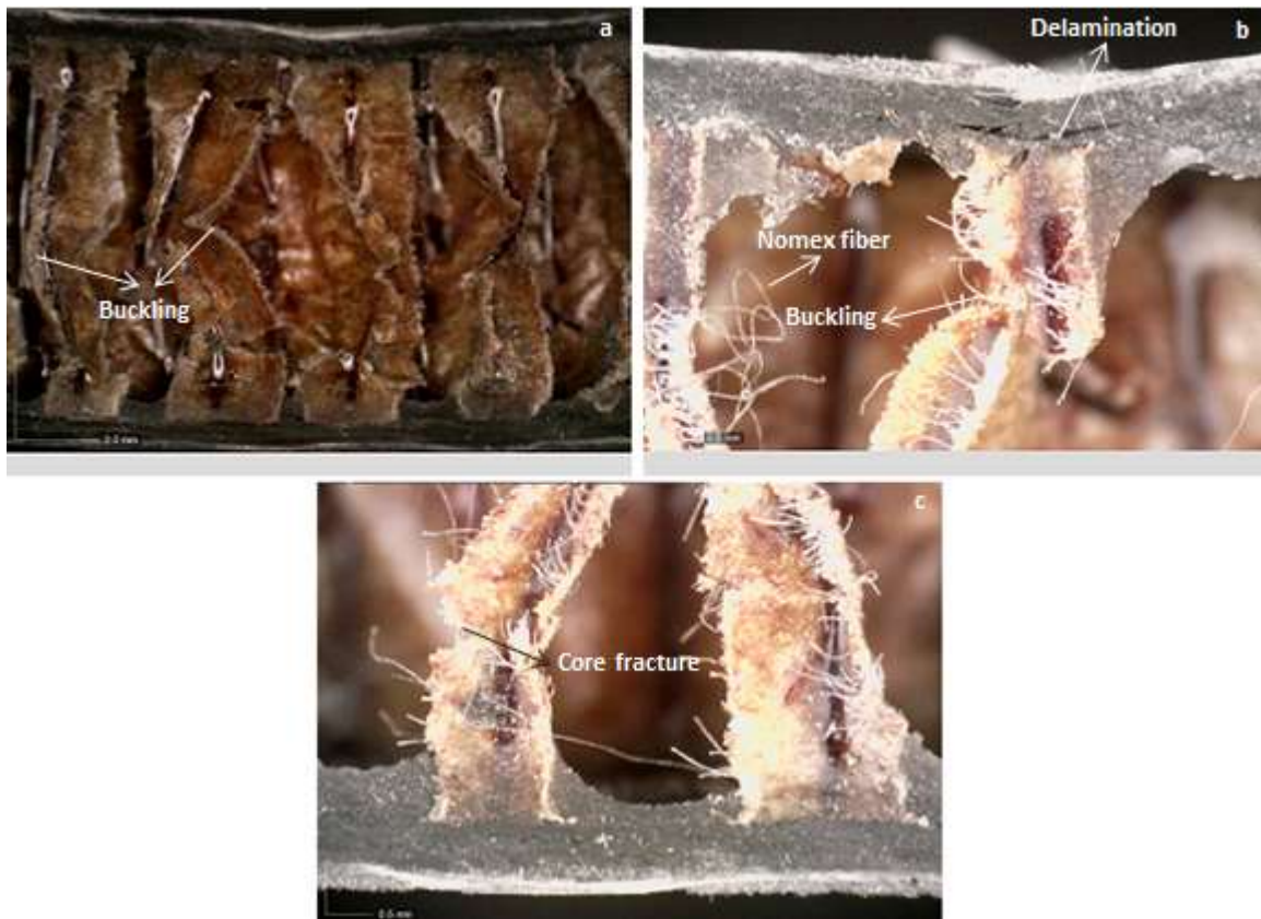
Figure 11. Micro images of 2C/1G/Nomex hybrid sample
