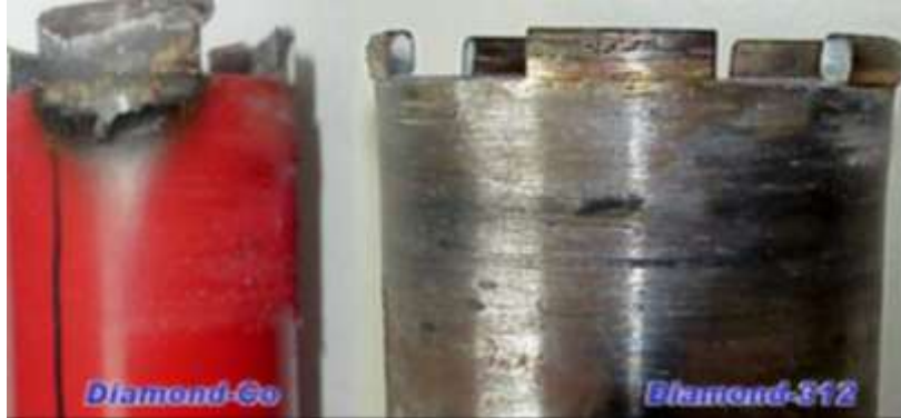
Figure 5. comparison of concrete dry drills made of diamond-Co and dimond-312 (Sun, 2011).
