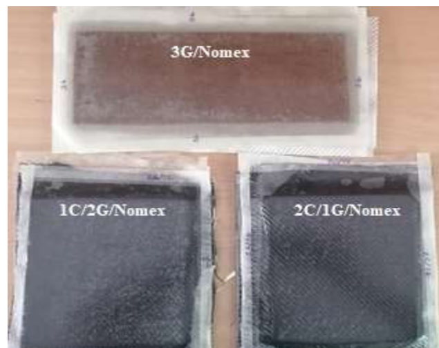
Figure 1. 3G/Nomex, 1C/2G and 2C/1G Hybrid/Nomex composite sandwich samples
